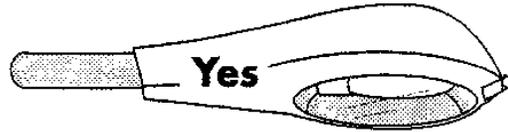
Flat glass lens, eliminates or minimizes direct glare, no upward throw of light. The housing for these fixtures are available in many styles.
